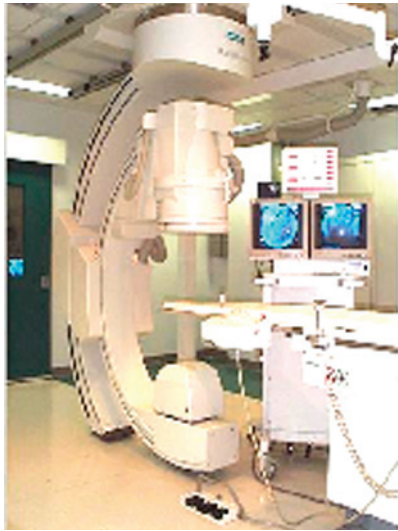
Figure 1. Modified Siemens Multistar rotational angiography prototype; the X-ray tube is located at the top position of the C-arm, X-ray image intensifier (XRII) is seen below. The C-arm rotates over 200° with a speed of 45° per second making acquisition times as low as 4.4 seconds.
